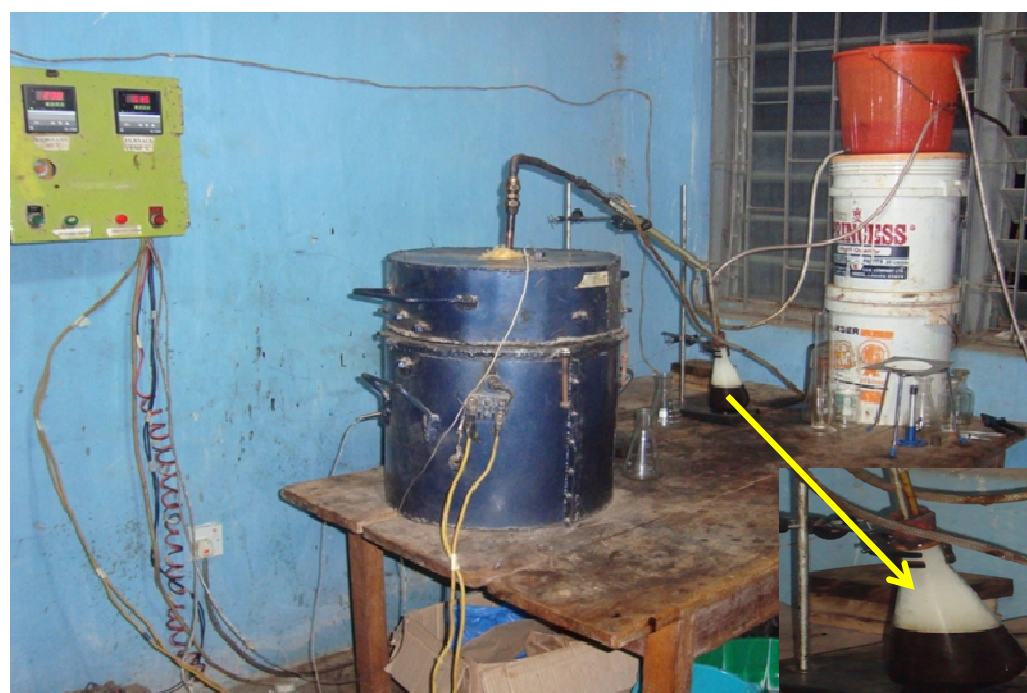
Fig. 1. Pyrolysis unit showing oil produced in a flat bottom flask
